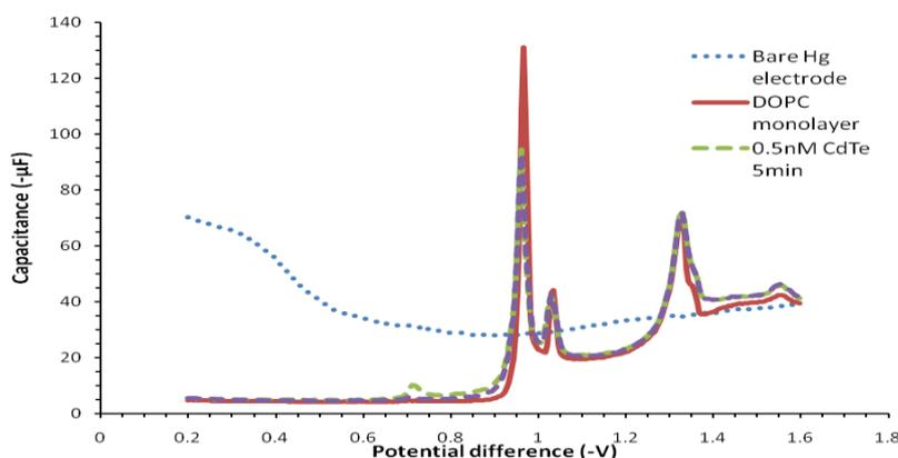
**Figure 1:** Capacitance versus potential profile of the bare Hg electrode, DOPC monolayer and CdTe cores over a period of 10 min at pH 7.4. Whilst some signal suppression by the CdTe cores is seen at -1 V, it is not significant enough to indicate interaction occurring. At  $\sim -0.7$  V a small peak is seen, which could be down to mercury redox or pore formation in the monolayer.
